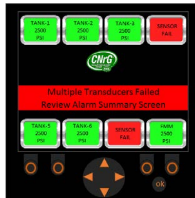
Figure 91. Multiple Pressure Transducer Sensors Unplugged/Faulty
