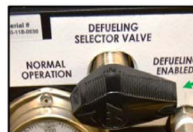
Figure 85. Fuel Module Defueling Selector Valve Set
