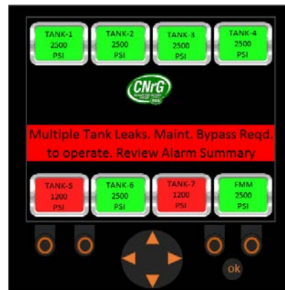
Figure 95. Multiple Tank Leaks. Maintenance Bypass Required.
