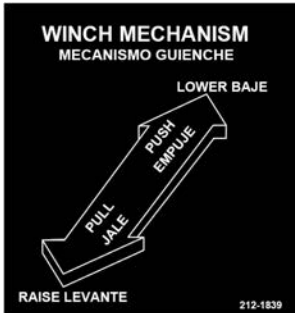
Figure 31. Winch Mechanism Controls, PN 212-1839
