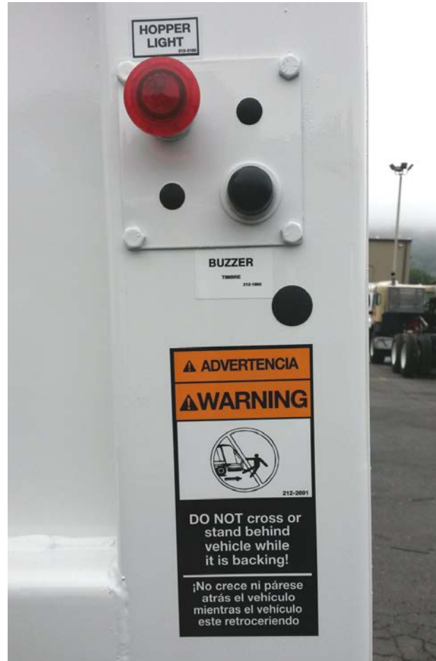
Figure 48. Buzzer and Hopper Light Switch Location
